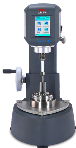
Figure 1: HAAKE Viscotester iQ Rheometer with Peltier temperature module and coaxial cylinder measuring geometry.
